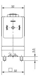
Cable plug DIN 43650, form A, (0-250 V AC/DC) delivery standard.
